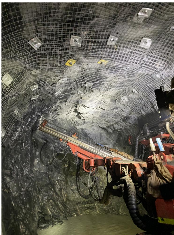
Figure 3 - Twin boom jumbo boring prior to firing the next Decline development cut
